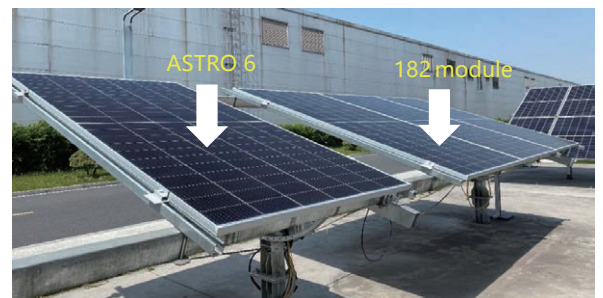
Project location: Haining, Zhejiang Province, China. Fixed tilt:20°, ground clearance:1.2m
